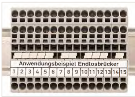
Continuous jumpers (2002 Series) readily connect an endless number of terminal blocks to each other via a single jumper slot. Use the second jumper slot for additional commoning or testing.
