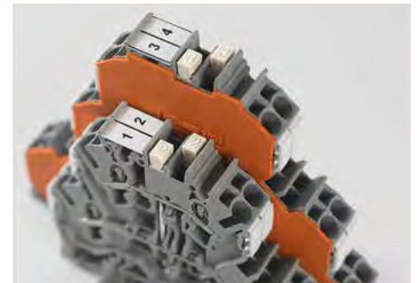
Created for double- and triple-deck TOPJOB® S Terminal Blocks, the vertical jumpers can common two or three levels. Clearly marked numerals ("2" and "3") distinguish the double-deck (2002-492) and triple-deck vertical jumpers (2002-493), even when inserted.
