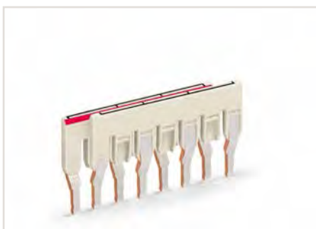
Staggering jumpers in a single jumper slot. When creating custom staggered jumpers (e.g., for bridging over a terminal block with a different potential), make sure that only one contact lug is in contact with the terminal block. The contact lugs of the customized staggered jumpers contact the terminal blocks via the gaps created in the second jumper. Insert and press the ready-made jumper assembly into the jumper slot until it hits backstop.
