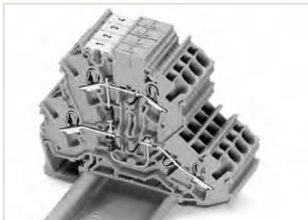
Double-deck diode terminal blocks were specifically developed for custom diode circuits, such as lamp test and collective fault signal circuits. These terminal blocks provide high-density wiring in a width of just 5.2 mm. Push-in type jumper bars provide additional options for custom circuit design.
