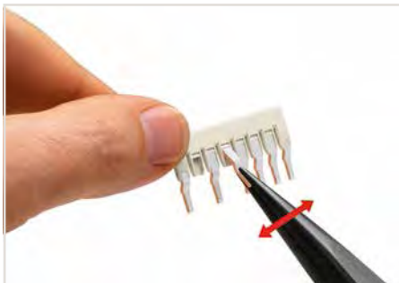
Staggered jumper (seven contacts) Individual jumper contacts can be broken off by bending them. The remaining piece of insulation will meet requirements for clearances and creepage distances.
