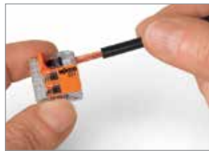
2. Open clamping unit using the lever and insert the conductor.
